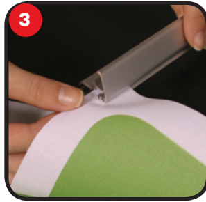
3 Insert graphic into graphic rails.
